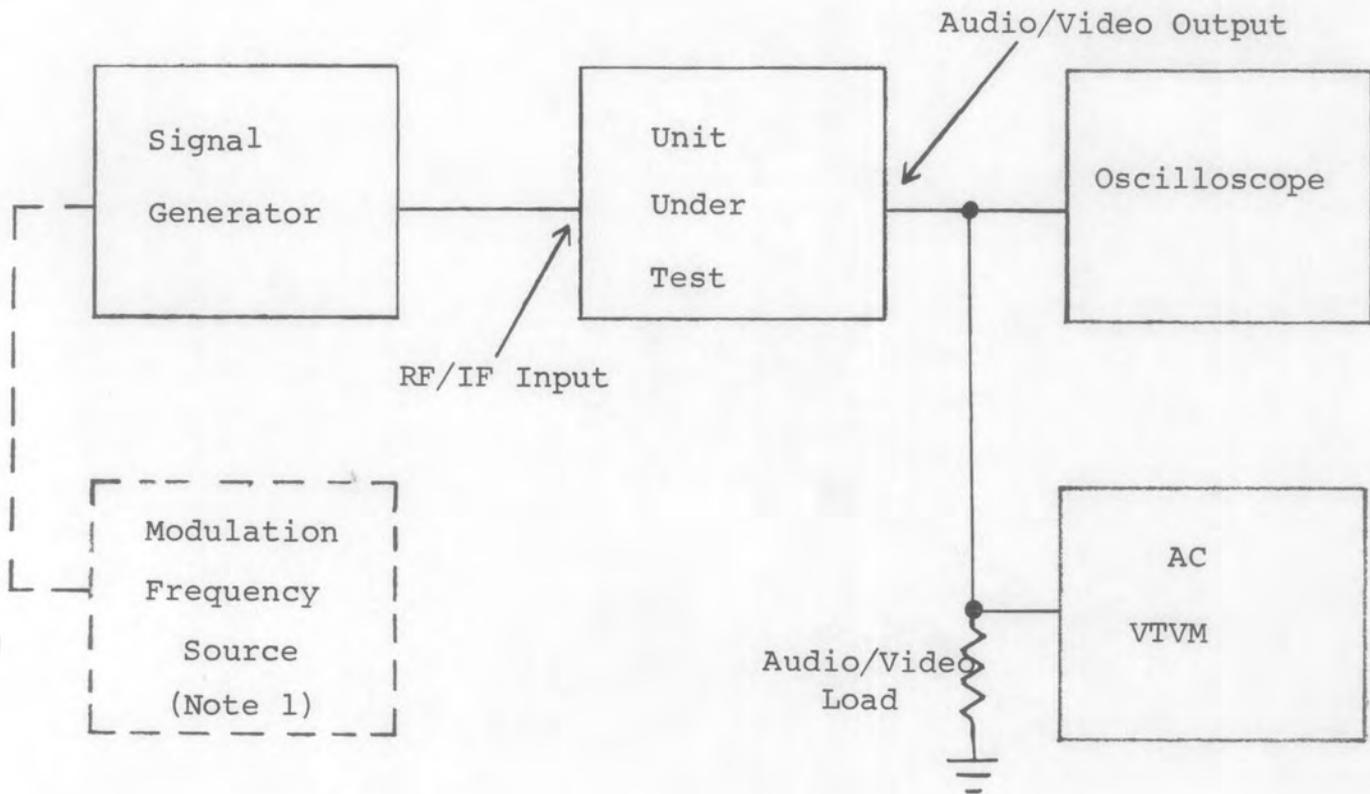
1. Set UUT to either AM/MAN, AM/AGC or FM/AGC reception/Detection mode. In AM/MAN mode, set RF/IF gain to maximum gain. Adjust tuned frequency of UUT to RF Test Frequency as called out in unit/equipment test procedure.
