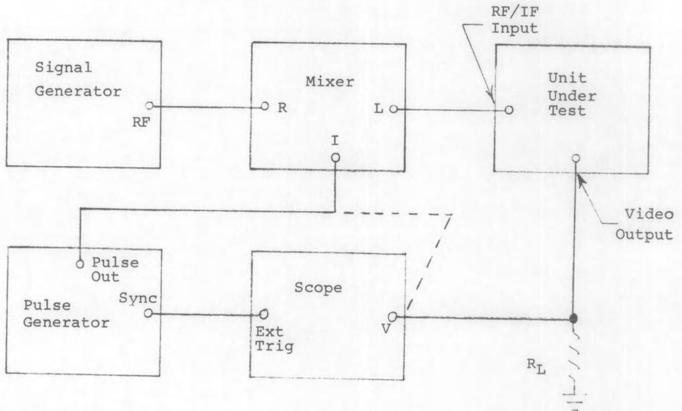
NOTE: For pulse lengths greater than 5  $\mu$ Sec equipment may be connected as shown in Standard Method 304-1.
