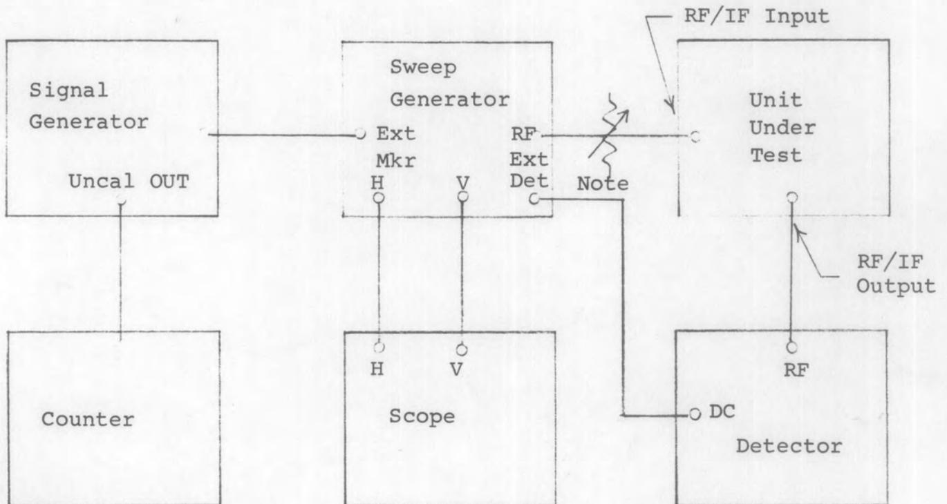
NOTE: Use an external attenuator if sweep generator output is not calibrated in dBm.
