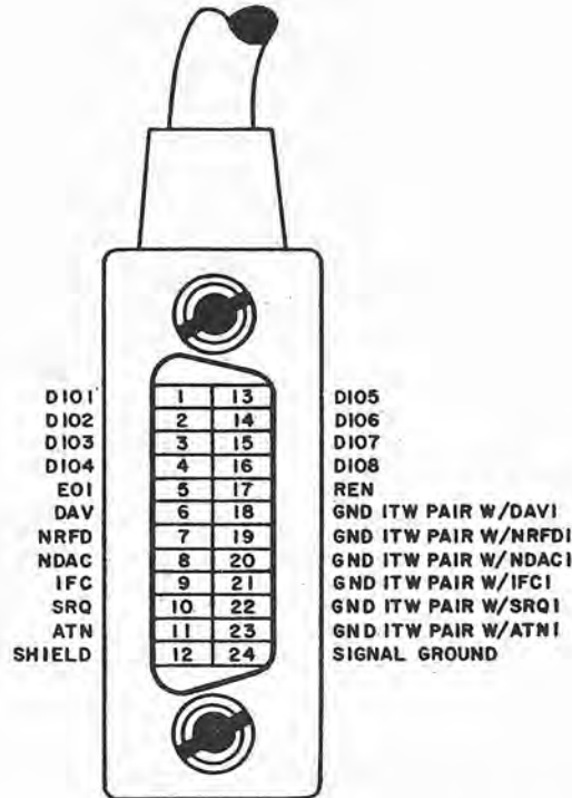
Figure 2-5. Configuration of IEEE-488 Data Bus
