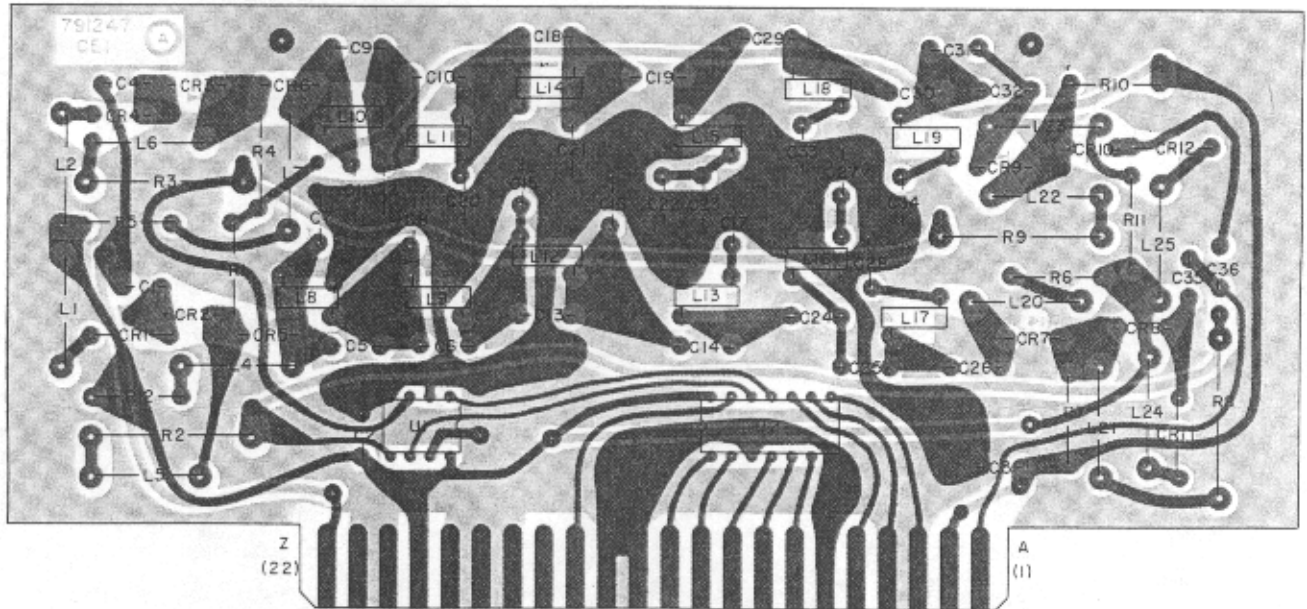
Figure 6-7. Type 791247 10-18/18-30 MHz Filter (A1A1A1), Location of Components
