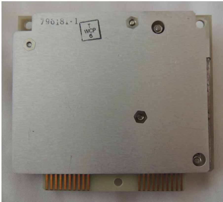
Figure 7a: The rear (shielded) side of the same 796181-X 10-Hz BFO Option card.
