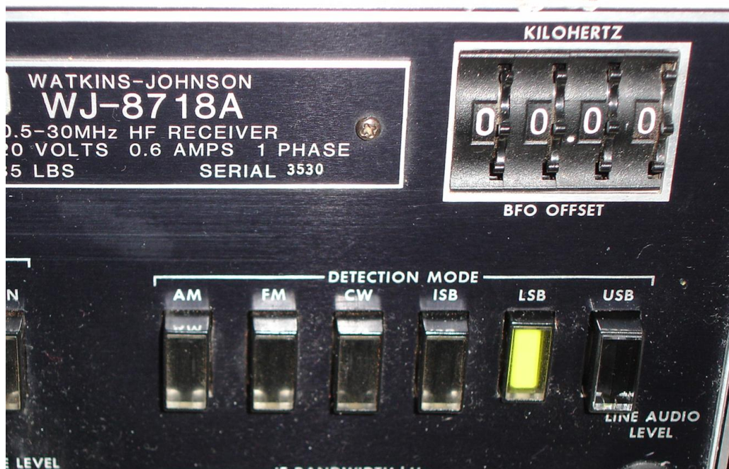
Figure 5: The four- section thumbwheel switch of a WJ-8718A provided with the 10-Hz BFO Option.
