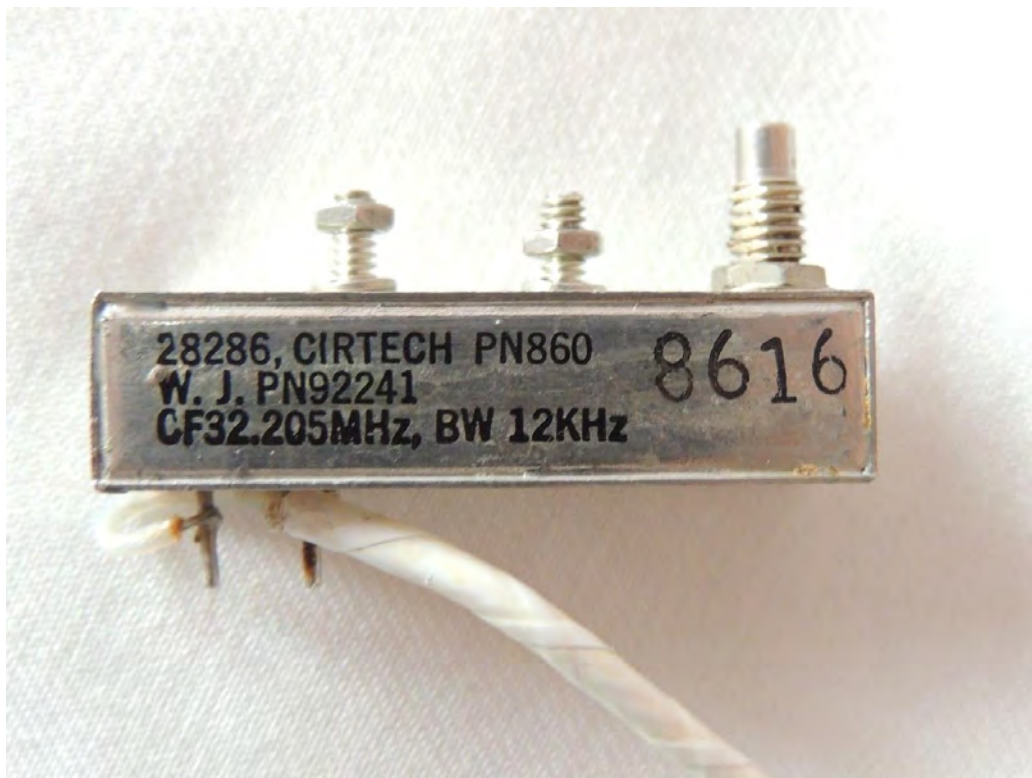
The FL2 32.205 MHz Xtal Filter used in later production units
