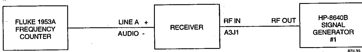
Figure 7-4. Fine Tuning Accuracy Performance Test Equipment Connection
