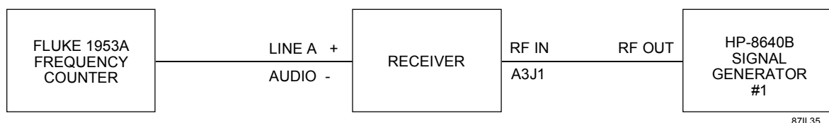
Figure 7-4. Fine Tuning Accuracy Performance Test Equipment Connection
