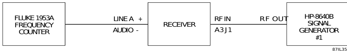
Figure 7-4. Fine Tuning Accuracy Performance Test Equipment Connection
