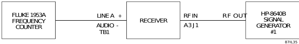
Figure 7-3. Fine Tuning Accuracy Performance Test Equipment Connection
