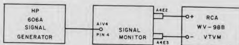
Figure 4-1. Equipment Setup, Interstage Alignment
