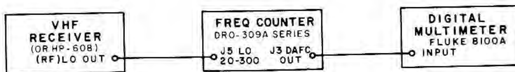
Figure 4-4. Equipment Setup for DAFC Range Test
