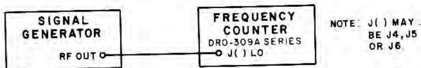
Figure 4-1. Equipment Setup for Count Input
