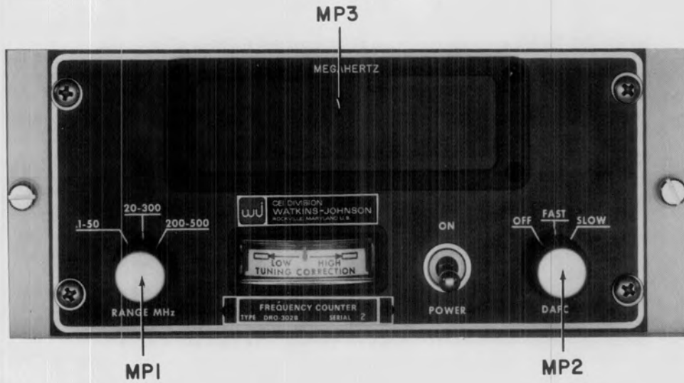
Figure 5-1. Type DRO-302B Frequency Counter, Front View, Location of Components
