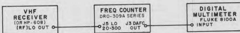
Figure 4-4. Equipment Setup for DAFC Range Test
