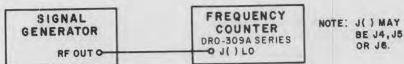
Figure 4-1. Equipment Setup for Count Input
