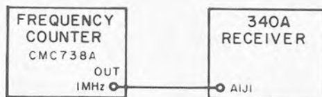
Figure 4-34. Test Setup, 1-MHz Oscillator Adjustment
