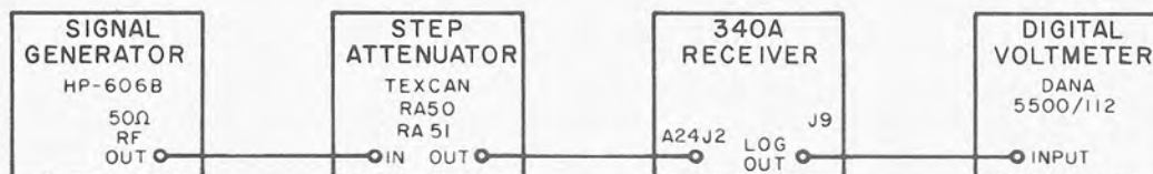
Figure 4-8. Test Setup, LOG Mode Operation Checks
