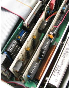
Figure 04: The Preselector Decode Card plugged in the X4 socket of the A6 mainboard.
