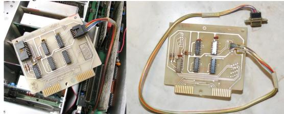
Figure 02: Two Preselector Decode boards with their multipole cable.
