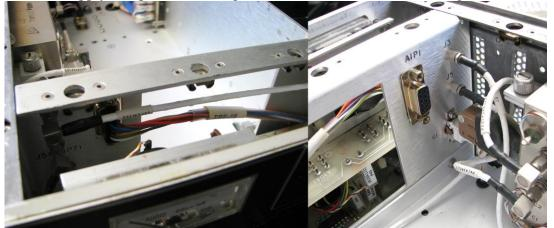
Figure 03: Routing the multipole cable in the receiver front (left picture) and installing the 9-pin sub-D connector in place (right picture). Please don't worry if your receiver is not provided with that large squared hole in the chassis, not all the WJ-8716/8718's have it!
