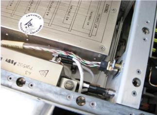
Figure 05: The Preselector 9-pin sub-D plug connected and fastened to its companion socket.
