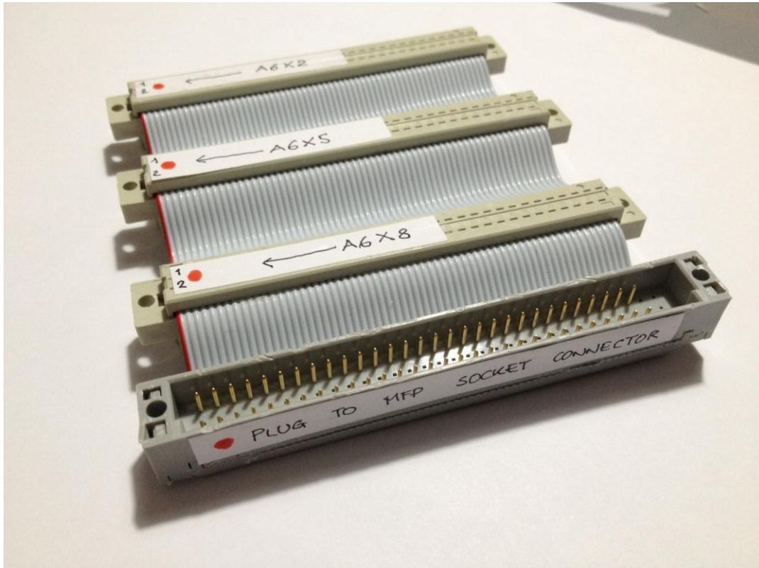
Figure 15: The correct final layout of the flat-cable jumpers with the male plug termination.
