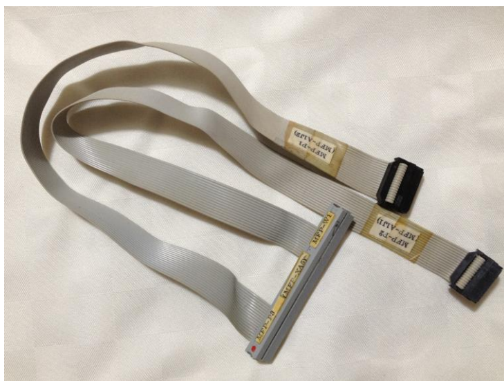
Figure 31: The MFP-W1 ribbon cable, splitted into two sockets at one end.
