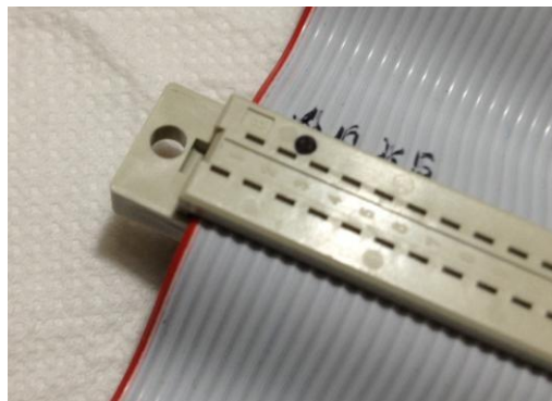
Figure 17: The pin numbers appear in the rear of the female sockets.
