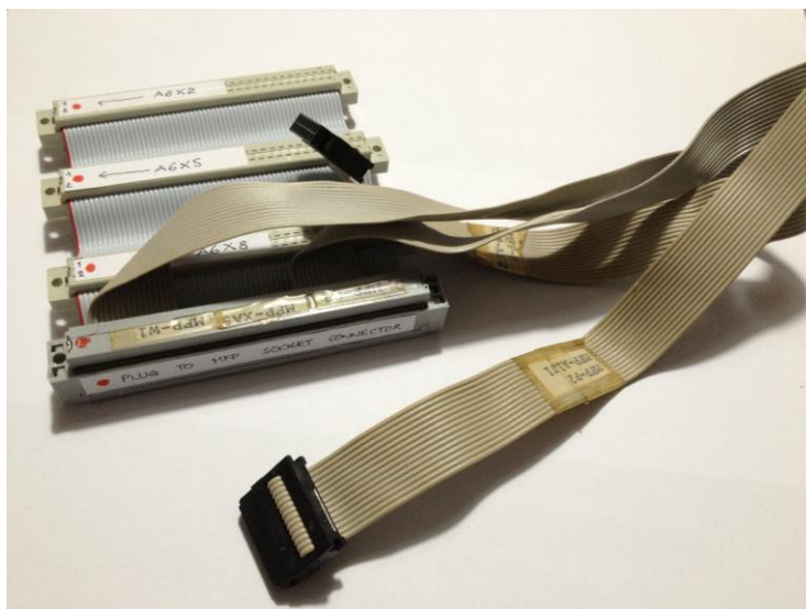
Figure 32: The MFP-XA5 64-pole socket inserted into the floating plug of the home-built ribbon cable assembly.
