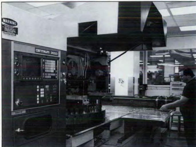
Executable CAD/CAM programs control precision cutting, bending, punching and milling processes to transform raw material into rugged, high-performance products.
