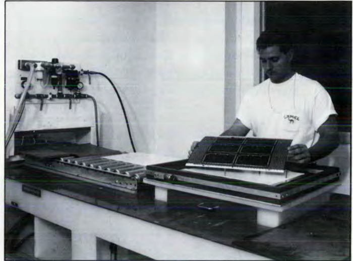
Fully equipped assembly shops and laboratories use both manual and automated fabrication techniques to etch, drill, cut to size and assemble single- and multi-layered printed circuit boards.
